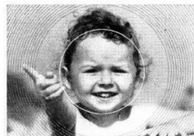
Microprism screen not fuzzy = sharp
