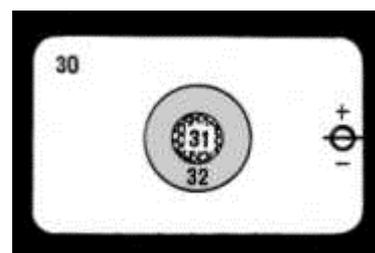
The ground glass circle is mainly used for micro- and macrophotography as well as for taking pictures with small apertures when microraster loses its sensitivity.
