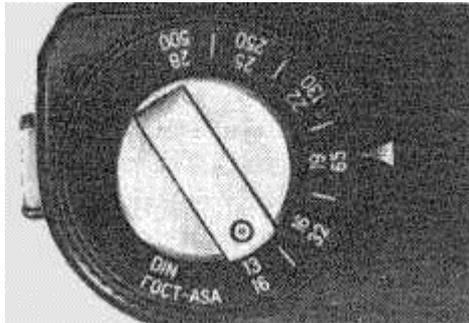
Semi-automatic exposure meter of your camera measures the light getting into the camera through the lens (TTL system). As a result you can set the exposure with the high degree of accuracy depending upon the brightness of the subject and the speed of photographic material by varying the shutter speed and aperture value.
