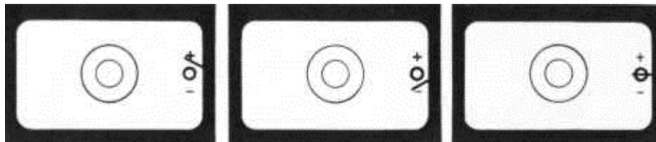
Watching in the viewfinder eyepiece in such a way that the whole of its frame would be clearly seen, press release button 3 till a definite stop but not till the shutter operation, should it be cocked.
