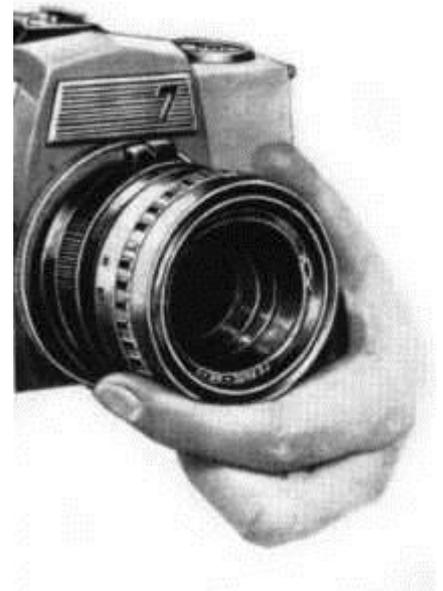
The depth of field is usually estimated with the help of scale 4 according to the distance scale. When it is necessary to estimate the depth of field visually, use ring 2. Having turned it fully to the right, it is possible to effect iris of the lens up to the earlier established value by hand. In this case on the ground surface you will obtain the image of such depth of field which corresponds to the set diaphragm value.
